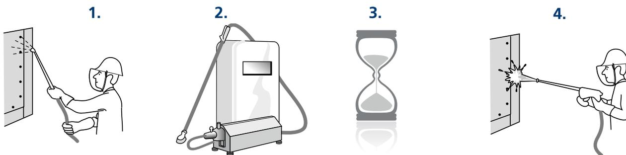
**1.1** To avoid smut formation after spray pickling, the passivator shall be applied before rinsing while the surface is still wet, "wet on wet". Leave the fluid to react 30 seconds.
